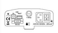
Attach the power supply cable to the connector on the rear of the analyzer. The master power switch is on the rear panel, next to the mains cable. Turn the power on.
