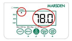
After a few seconds the scale will lock on the person's weight. When the patient leaves the scale, the weight will remain on the display.
