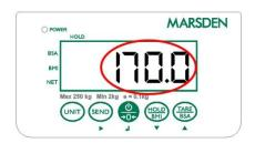
Hold down the HOLD/BMI button to enter BMI mode. The scale will enter height setting mode and the extreme left digit will flash.
