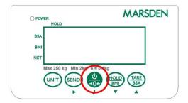
Press the ON/ZERO/OFF button firmly.
