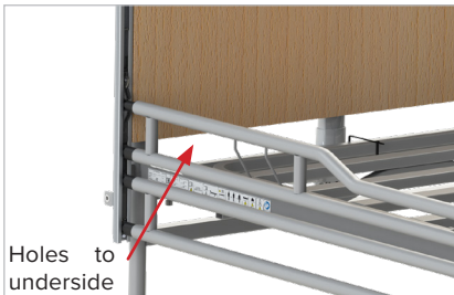
8.6.7 Bottom side rail inserted
