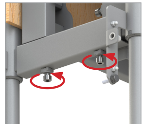
8.1.3 Bottom grub screws on the transport stand
