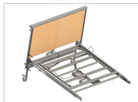
8.2.3 Bed end and backrest section assembled
