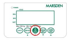
Hold the ON/ZERO/OFF button for three seconds when the scale is turned on. The scale will power down.
