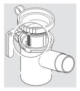
Attach the connection tubing to the nebuliser.
