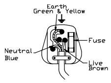
If you fit your own plug and the colours of the wires in the mains lead do not correspond with the markings identifying the terminals on your plug proceed as follows:-
